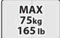
(EN) Do not exceed the maximum load specified for the roof rack, accessory rack or the maximum load recommended by the vehicle manufacturer. **Max roof load = weight of the complete roof rack system + weight of the load**
