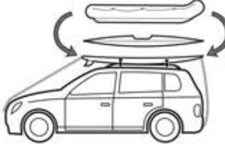
(EN) Any load extending over the windshield (except roof baskets) must be secured to both the front and rear of the vehicle, in addition to the rack. Failure to do so may result in property damage, personal injury or death.
